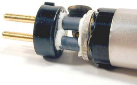
Figure 15 – Ferrite beads protect a microphone
