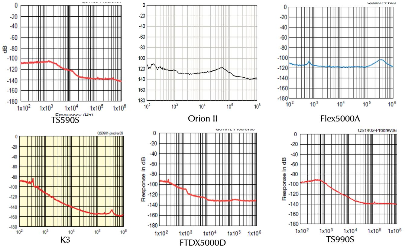
Figure 11 -- Selected Raw ARRL Lab Phase Noise Data
