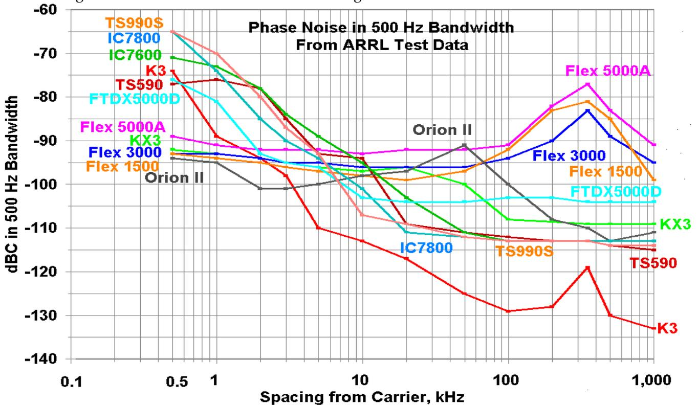
Figure 10 – Phase Noise Either Side of a Carrier
